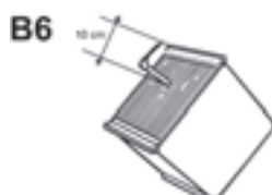
B6 MOISTURE ROD INSTALLATION
