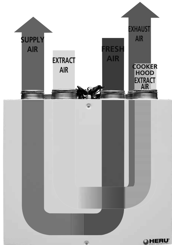
LEFT HANDING APPLICATION: HERU®70 T, 100 T EC, 160 T EC (WITH OR WITHOUT COOKER HOOD CON.). HERU®200 T EC, 250 T, 250 T EC (EXCEPT COOKER HOOD CON.).
